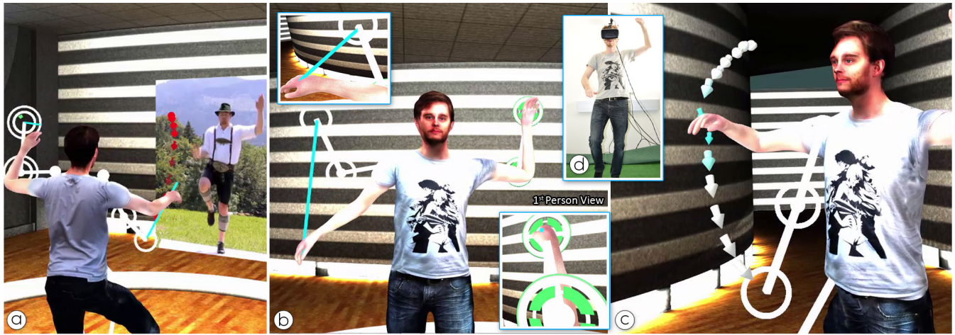
Figure 1: Prototype system for Study 1: (a) Motion guidance around the lifelike avatar. (b) Blue rubber bands indicate links between the desired posture and the user pose, the highlighted glyph indicates when posture is completed. (c) Arrows show the motion path and an animated stick figure is used for postures. (d) User during the study, wearing the Oculus Rift HMD.
