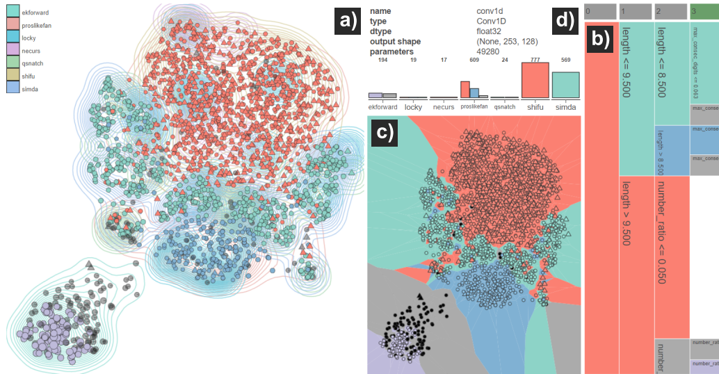
Figure 1: The analysis view for the first convolutional layer of the CNN (for domains with length in [8, 10] and top-level domain eu): a) 2D projection of the activations, displaying cluster and class membership. b) Calculated decision tree for the cluster labels, which uses length as the primary separator. c) Voronoi diagram of the 2D projection, showing the separation in the last decision tree level. d) Layer information and per-class cluster distribution.
