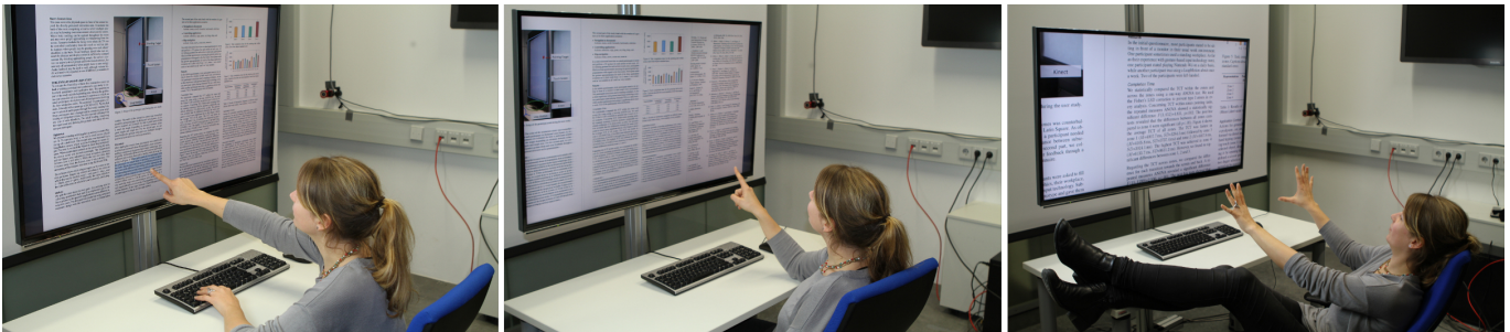
Figure 1: Providing seamless proxemic interaction for document reading: users perform text selection through touch (left), flick through pages using fine-grained finger-gestures (middle), and zoom from afar using coarse hand gestures (right).
