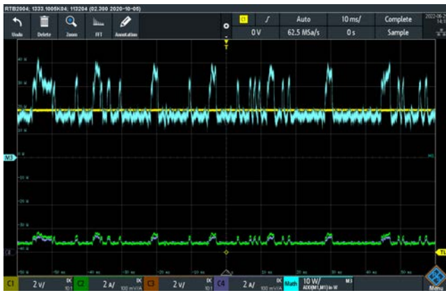
Figure 5: Measurements of the voltage and current probes of an oscilloscope attached to the PCIe cables of an NVIDIA RTX 3090 while performing a volume rendering task. The odd-numbered probes C1 and C3 are the voltage probes, whereas the even-numbered ones C2 and C4 are the respective current clamps. The cyan-coloured math chart is the combined apparent power of both power lanes.
