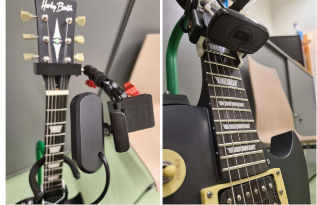
Figure 6: Color cameras are attached rigidly to the guitar. One camera is mounted on the guitar’s headstock oriented towards the guitar’s neck (left), while a second camera is mounted on the fretboard, to capture the strumming (right).
