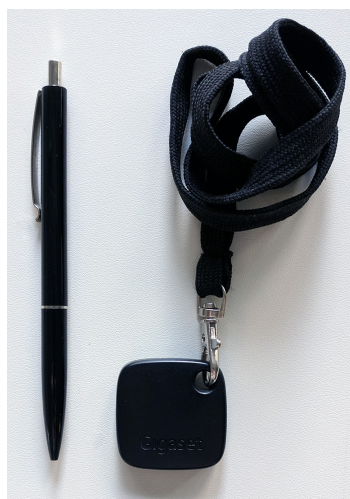
Figure 7: A Bluetooth Low Energy (BLE) beacon as used in the study. All participants carried the same type of beacon, allowing for a reliable detection of nearby users. Ballpoint pen for scale.
