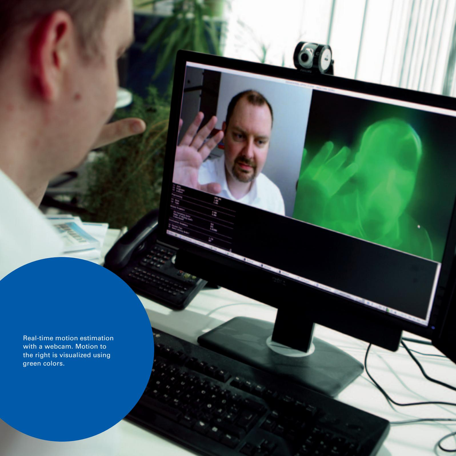
Real-time motion estimation with a webcam. Motion to the right is visualized using green colors.
