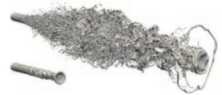
Visualization of planar patches that are used to approximate the fluid interface in the two-phase flow simulation.
