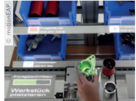
Working station that uses motionEAP technology to display projected assembling feedback as a work assistance.
