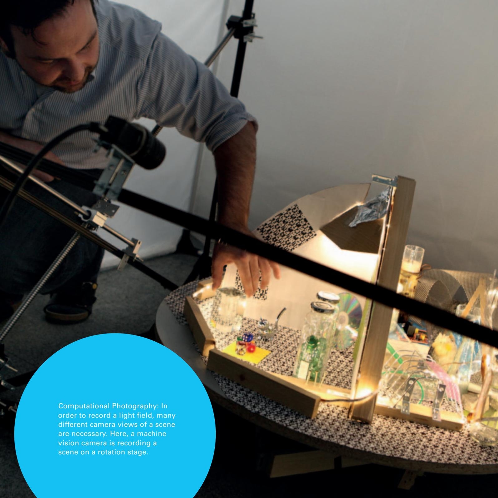
Computational Photography: In order to record a light field, many different camera views of a scene are necessary. Here, a machine vision camera is recording a scene on a rotation stage.
