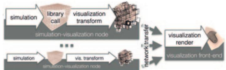
An integral part of this process are the intermediate visualization representations, which usually not only allow for reduced cost for storage and transfer but also for image synthesis.
