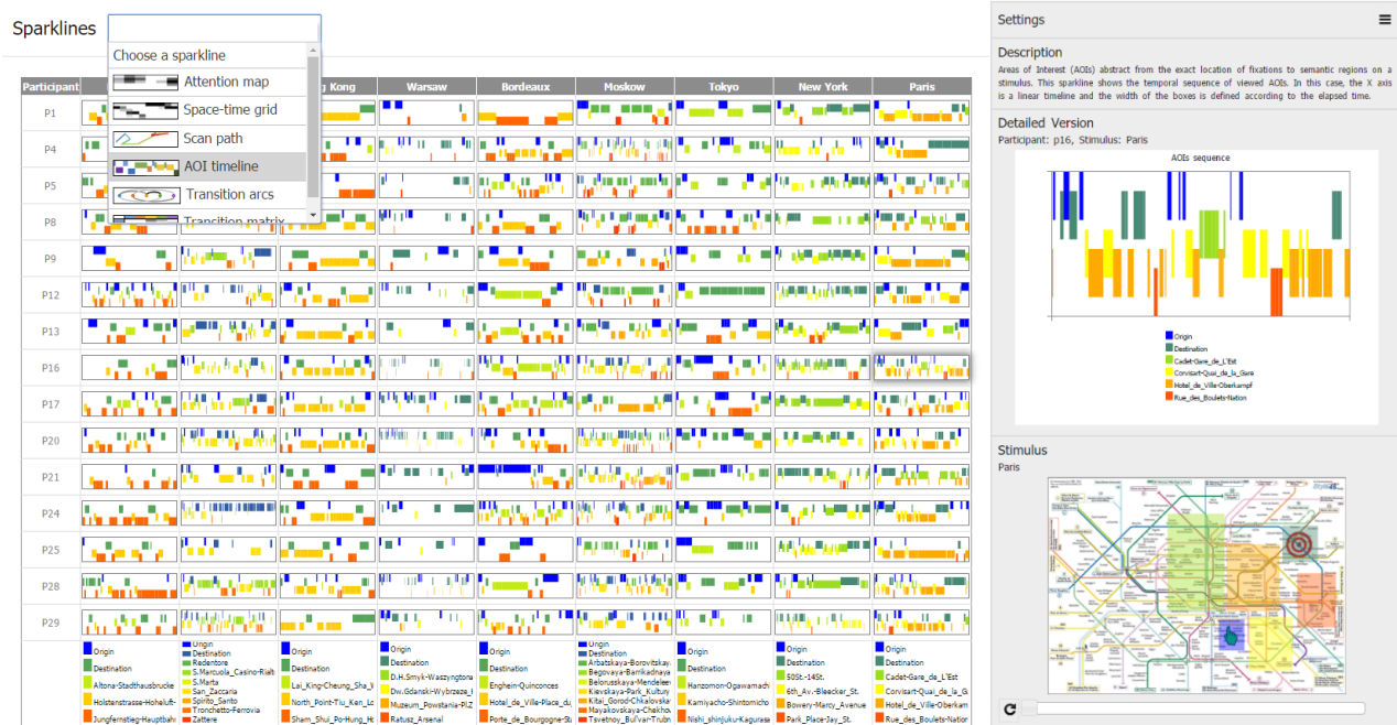
Figure 1: Analysis framework depicting eye movement data for different stimuli (columns) and participants (rows) in a tabular grid as word-sized visualizations. An analyst can choose between different variants of visualizations. On selection of a cell, the framework provides details such as a description, an enlarged version, and the original stimulus.
